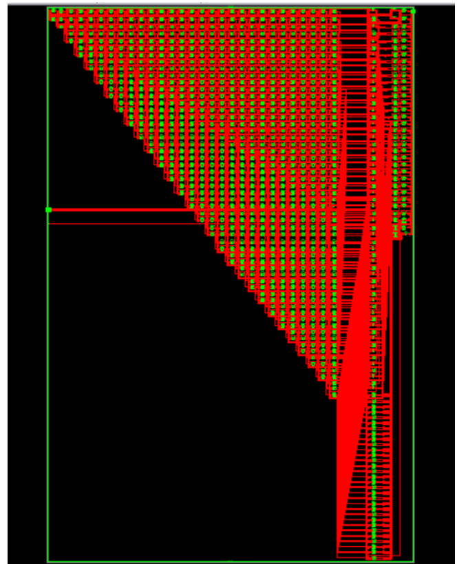
Fig-11: RTL Schematic of Wallace Tree Multiplier (CSA)
