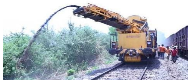
Fig.2 Conventional type large deep screening machine
