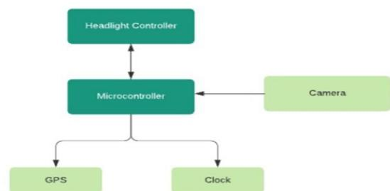
**Fig. 2. Flow of data to Headlight Controller**
