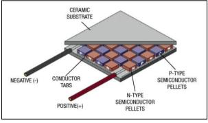
Fig.2 (b) Internal construction of Thermo-Electric Module
