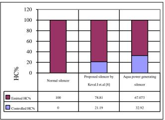
Fig.10 Comparison of HC reduction between Aqua power generating silencer and the silencer proposed by Keval.I et.al [8]
