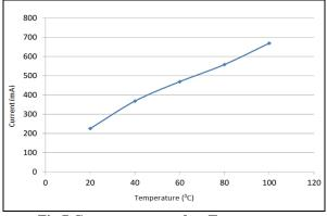
Fig.7 Current generated vs Temperature
