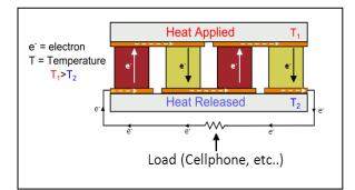
Fig.2 (a) Thermo-Electric Module
