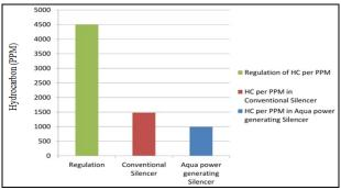
Fig.5 Comparison of HC (ppm) in exhaust emission between Conventional and Aqua power generating silencer
