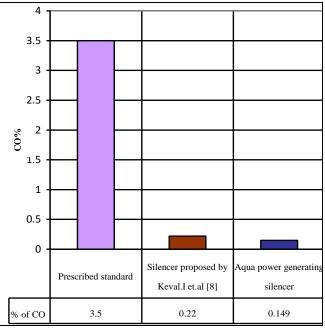
Fig.9 Comparison of CO reduction between Aqua power generating silencer and the silencer proposed by Keval et.al[8]
