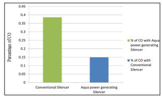
Fig.4 Comparison of CO (%) contained in exhaust emission between Conventional and Aqua power generating silencer
