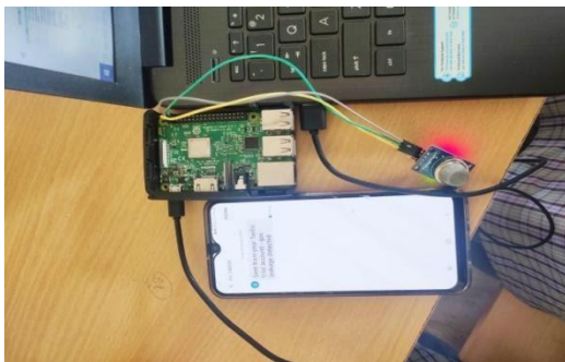
Fig5: Gas leakage detection
