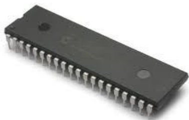
Fig 5 PIC 16F877A Microcontroller
