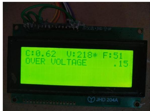
Fig. 8. Overvoltage condition
