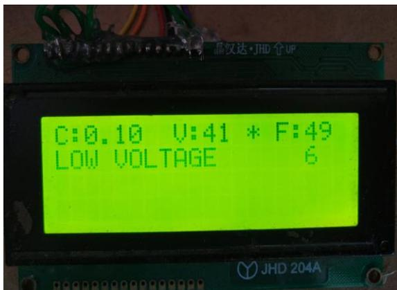
Fig. 9. Undervoltage condition
