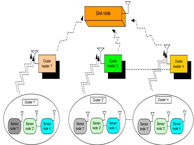
Fig.1. WSN architecture-based water level regulation
