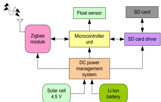
Fig.2. Sensor node with power management
