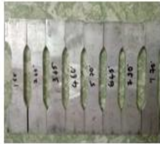
Fig 2: Tensile test pieces
