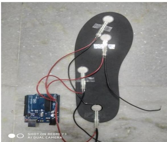
Fig. 3. Insole FSR Sensor System
