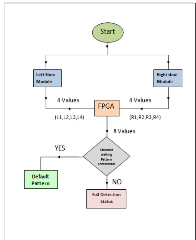
**Fig. 5. Flow Chart for Proposed Algorithm**
