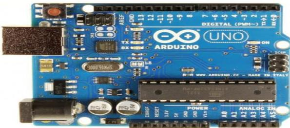
Fig.3. Arduino Uno board
