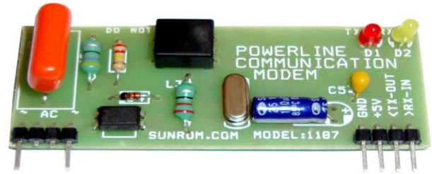
Fig.4. Front View of the Modem
