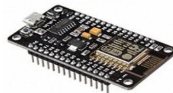
Figure 4: NodeMCU with ESP8266 Wi-Fi chip
