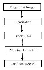
Fig 4.4 Fingerprint Authentication Process Diagram. [2]
