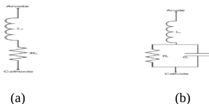
Fig.1.1. PIN-diode identical circuit (a) ON state (b) OFF state
