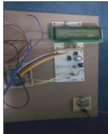
Fig 4.2 Fire Sensor Connected to Arduino.
