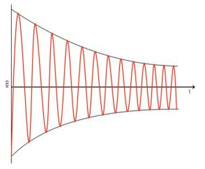
Fig. 2. AC Symmetrical short circuit current waveform
