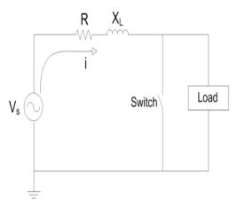
Fig. 1. AC Symmetrical fault current circuit diagram
