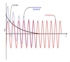
Fig. 4. Total (DC and AC components) short circuit AC symmetrical current
