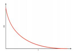
Fig. 3. DC offset short circuit current when decaying
