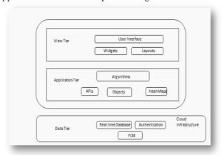
Fig. 2. System Architecture for Mobile Application
