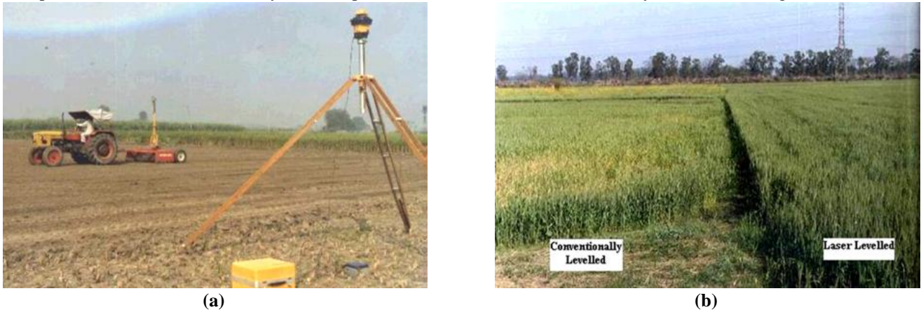
Fig. 1(a & b). Laser land leveller in operation and comparative crop performance of laser and conventional land levelling.
