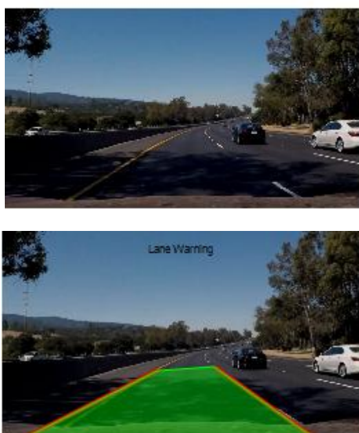
Result (4): Frame with missing marking and 'Warning' for lane departure
