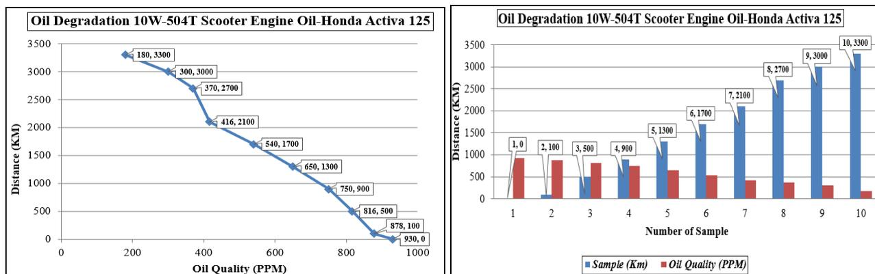
Fig. 12. Oil Degradation 10W-50 4T Scooter Engine Oil-Honda Activa 125
