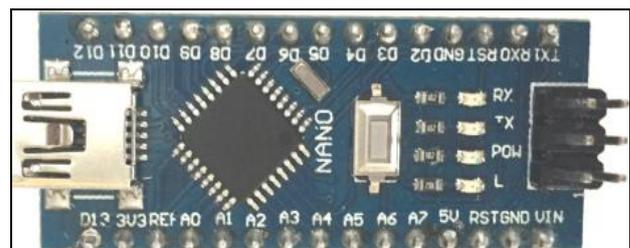
Fig. 6. MCU (Arduino NANO) [10]
