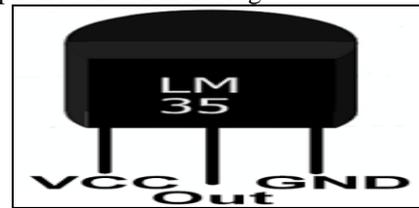
Fig. 4. LM35 Temperature Sensor [3]
