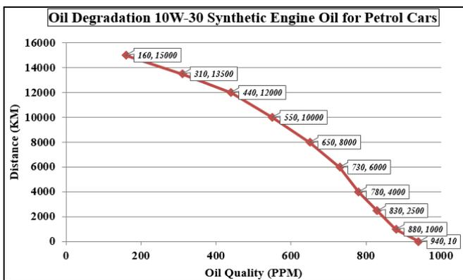
**Fig. 15. Oil Degradation 10W-30 Synthetic Engine Oil for Petrol Cars**
