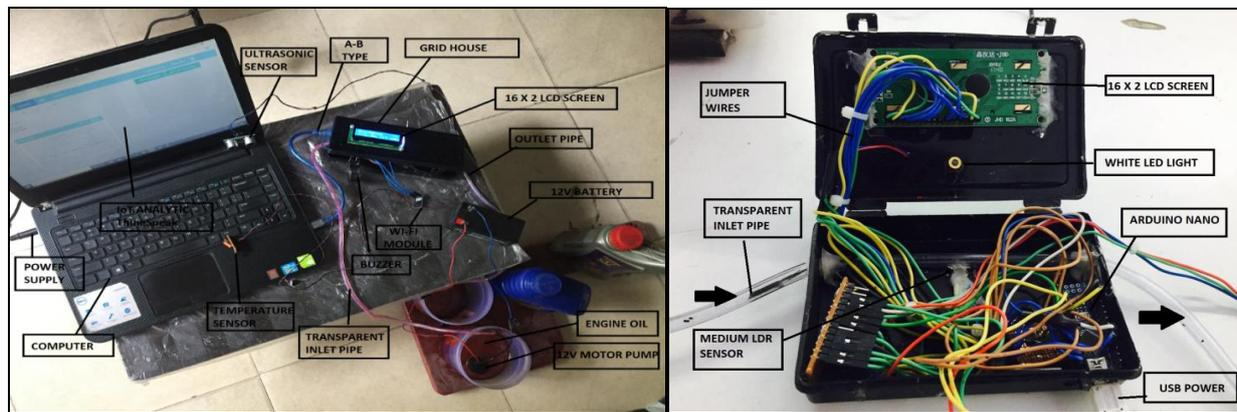
**Fig. 10. Developed EOM System**
