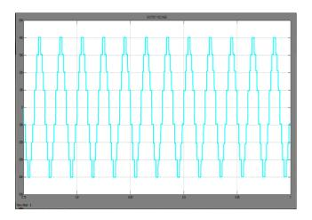
Fig 6.5. Proposed Nine Level Output Waveform
