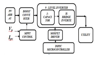
Fig: 1 Block Diagram of Proposed System
