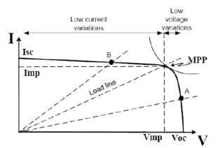
Fig 3 Graph with Voltage and Current
