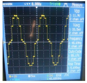
Fig. 7.2 Output voltage of nine level inverter
