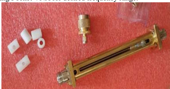
Figure 3: Fabricated 50 ohm Impedance tuner with derlin runners
