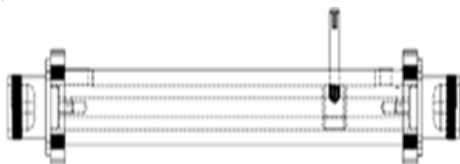
Figure 2: Brass tuner design for fabrication
