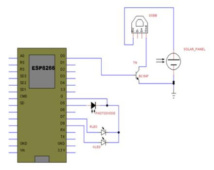
Fig. 3 Circuit diagram of Receiver
