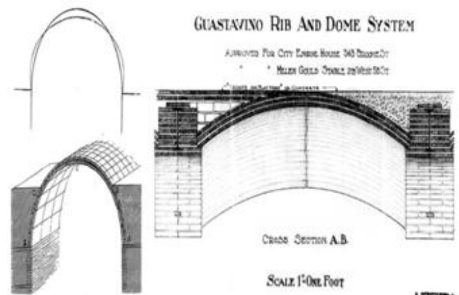
Fig.2 tile vaults with filling material. (left) descriptive drawings by choisy (1873); (right) guastavino rib and dome system [3].
