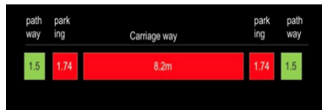
Fig 6. Existing Road width (red) and widened area (green)
