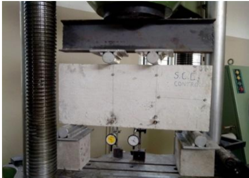
Fig.4 shows the testing of the beam
