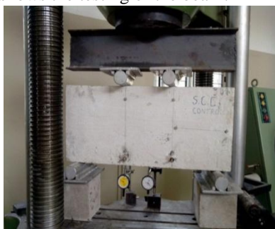
Fig.4 shows the testing of the beam
