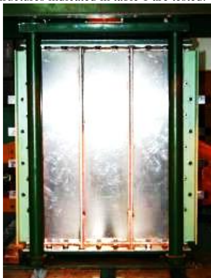
Fig. 4: Collapse testing of composite panels
