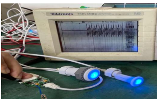
Fig. 9. Set up showing the LED powered by WPT
