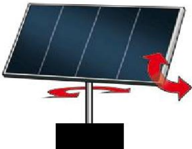
Fig. 2. Dual Axis Solar Tracker System [6]
