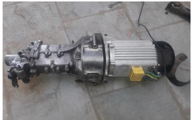
Figure.7. Coupled motor with gearbox
