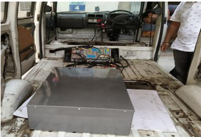
Figure.10. Final assembly of drive train
