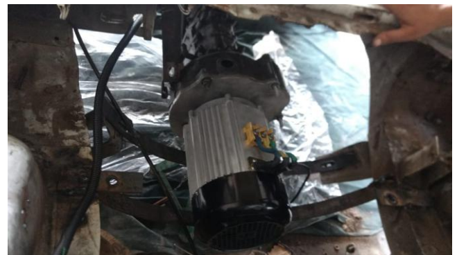
Figure.8. Mounting of motor coupled with gearbox
